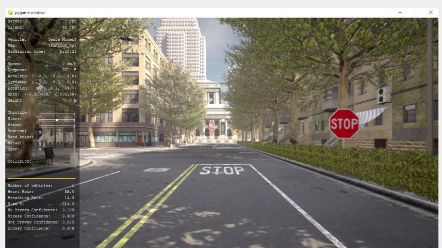
Fig. 2: CARLA displaying driver's biometrics, vehicle controls and model confidence values.
