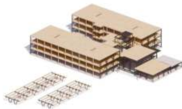
HYBRID STRUCTURAL SYSTEM: MASS TIMBER WITH EXPRESSED STEEL BRACE FRAMES
