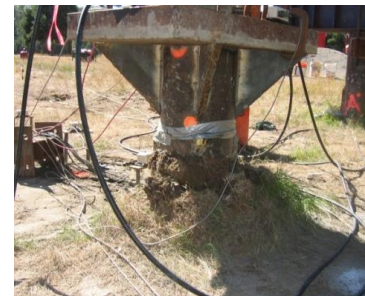
Photos showing liquefaction induced settlement of 11 inches around the test pile that
