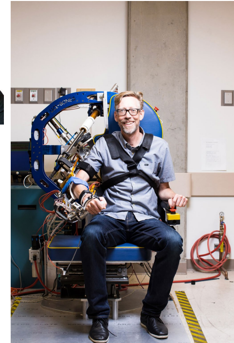
David Reinkensmeyer demonstrates one of his robotic devices created to help patients recover hand and arm function after neurologic damage caused by stroke or spinal cord injury.
